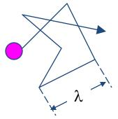
$\begin{aligned} \tau_{\rm c} &= \text{average time between collisions} \\ \lambda &= \text{mean free path} = v_{\rm th} \tau_{\rm c} \\ \tau_{\rm c} &= 10^{-13} \text{ sec, so } \lambda = 10^5 \, \text{x} 10^{-13} = 10^{-8} \text{m} = 10 \text{nm} \end{aligned}$
